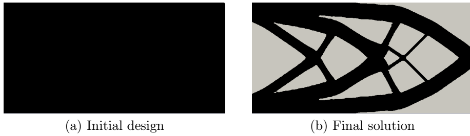
Figure 13: Initial design and optimal solution for the cantilever example.
