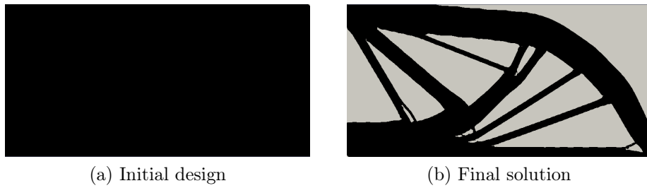
Figure 16: Initial design and optimal solution for the MBB example.
